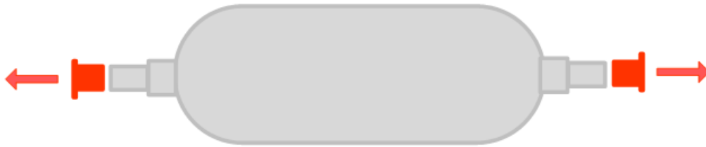
Figure 5 - Open locking caps of the ICR
