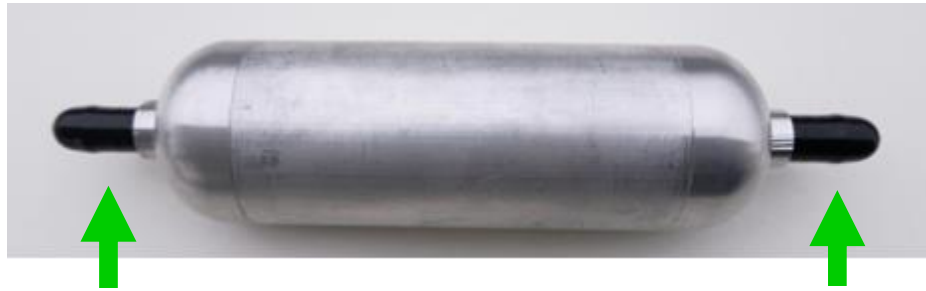
Figure 2 - ICR - arrows point to locking caps
